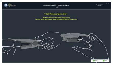
Then after clicking continue, you will be directed to the photoplethysmograph (PPG) sensor functionality checking page so that there are no errors in the data collection process.
